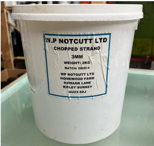
Chopped Fibre Glass Strand, 3mm for reinforcing refractory molds, 1.5kg left - £7.50
